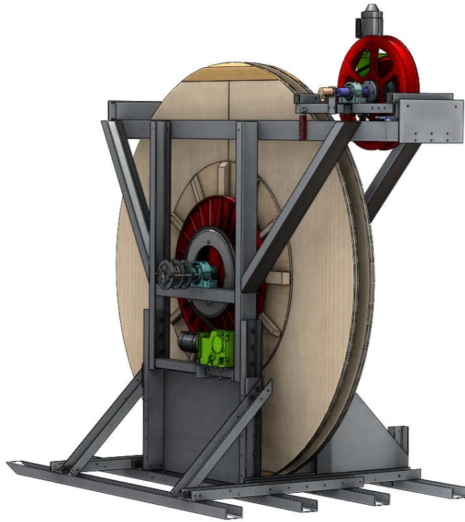
Figure 24: Antarctic Rodwell Apparatus Return Water Cable/Hose Reel. This design accommodates the usage of a bundled cable that carries power and signal. This allows the design to be compact enough to integrate onto the Tower Operations Site Air Ride Cargo Sled.
