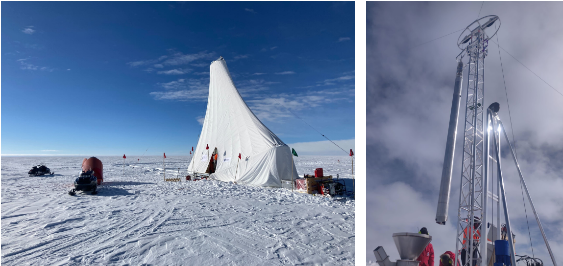
Figure 38: BigRAID Drill as used at RNO-G in field-season 2022. Left: during operations, the drill rig is covered by a tent to prevent ice forming on the barrel and protect the drill crew from the environment. Right: The drilling barrel raised on the tower.
