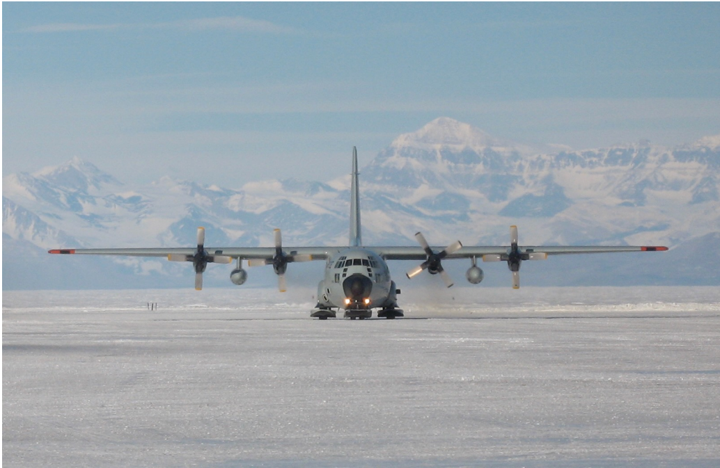
Figure 45: Ski-equipped LC-130 "Hercules" of the New York Air National Guard in McMurdo. Image: Albrecht Karle, IceCube/NSF
