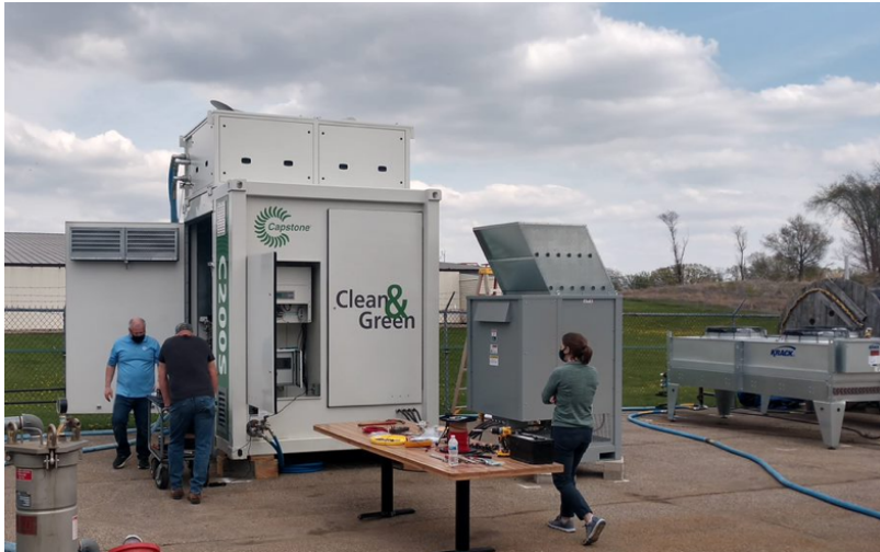
Figure 7: A Capstone CS1000S microturbine has been purchased by PSL and is currently being used for research and development and testing in support of IceCube-Gen2. The microturbine is currently installed in the PSL testbed.
