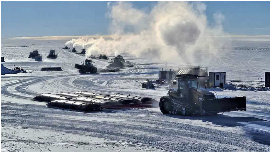
Figure 46: South Pole Traverse (SPoT) delivering fuel and materials to the South Pole. The nearer tractor is towing sleds with fuel bladders.
