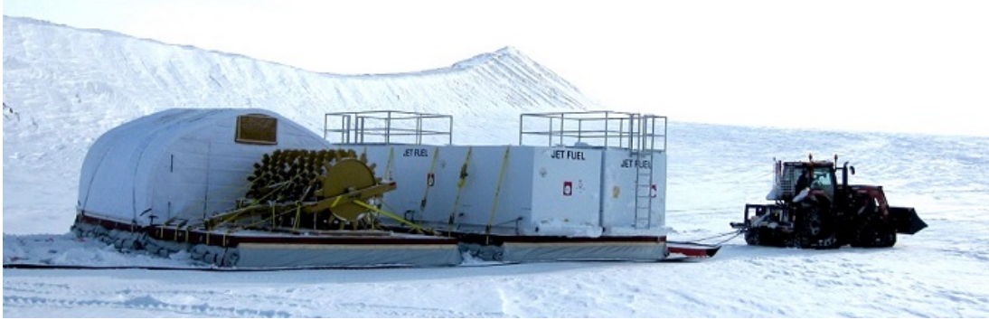
Figure 19: ARCS carrying two 25,000-lb steel fuel tanks and a 14,000-lb roller-packer for an outbound trip from Thule to Summit Station.
