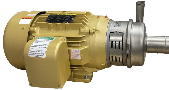
Figure 16: An SPX Flow centrifugal pump will transfer water up to 80 GPM and 115 to 140 PSI from the hot water tank to the HPP. The pump is shown attached to a 50 horsepower Baldor motor.
