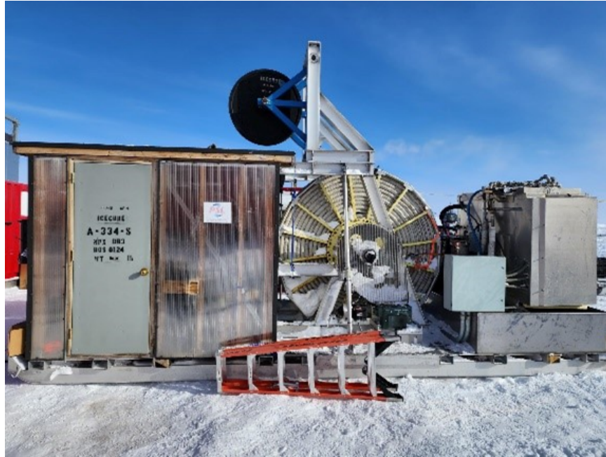
Figure 31: The Independent Firn Drill (IFD) shown in service at the South Pole.
