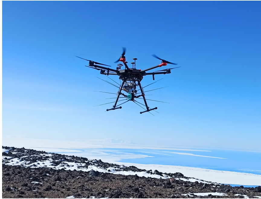
Figure 137: Drone Pulser used for TAROGE-M experiment, and proposed for IceCube-Gen2 radio.
