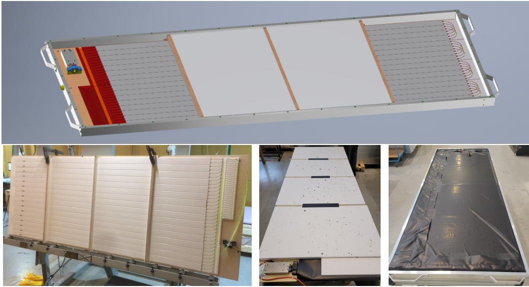
Figure 95: Schematic (top) and photos (bottom) of the assembly of a scintillation detector, from left to right: routing of optical fibers through the scintillator bars of the detector to the cookie that interfaces to the SiPM; Styrofoam cover of the scintillator bars; light-tight foil cover. In a final step not shown in these photos, the scintillation detector is closed by an aluminum sheet.
