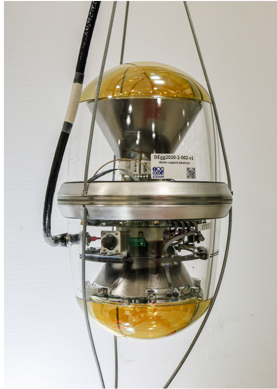
Figure 78: A D-Egg module designed and built for the IceCube Upgrade. The D-Egg sensor is sealed in the UV-transparent glass housing with the waistband around the equator. Each PMT is carefully fixed in place in either an upper or lower glass hemisphere by using a UV-transparent optical coupling gel. Inside are the electronics mainboard, calibration devices (cameras, LED flashers), and magnetic shielding.
