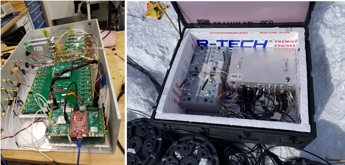
Figure 86: Instrumentation boxes (left: DAQ box in lab, right: vault in field) of RNO-G, for illustration purposes. The DAQ box for IceCube-Gen2 will be built as shown schematically in Fig. 85 and Fig. 88. In the field, the metal DAQ box is in an environmental enclosure with cable feedthroughs for power, communication, and signal cables. The IceCube-Gen2 vault will be smaller since the stations will not require batteries.
